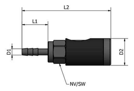
D1 ((mm) = Ø6 D2 (mm) = 26 L1 (mm) = 25 L2 (mm) = 88.5 SW (mm) = 21 Weight (g) = 110
